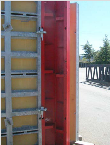
View of Inside Articulated Corner connected to Sterling Panel with Wedge Clamps.
